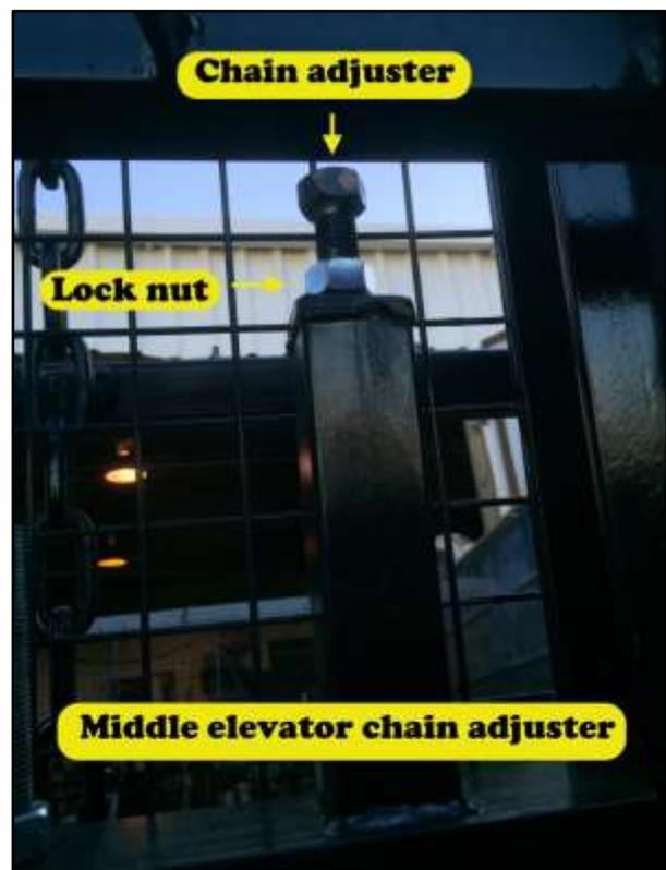
**Tip:** These chain adjusters have a M20 thread and require a M30 spanner/socket.
