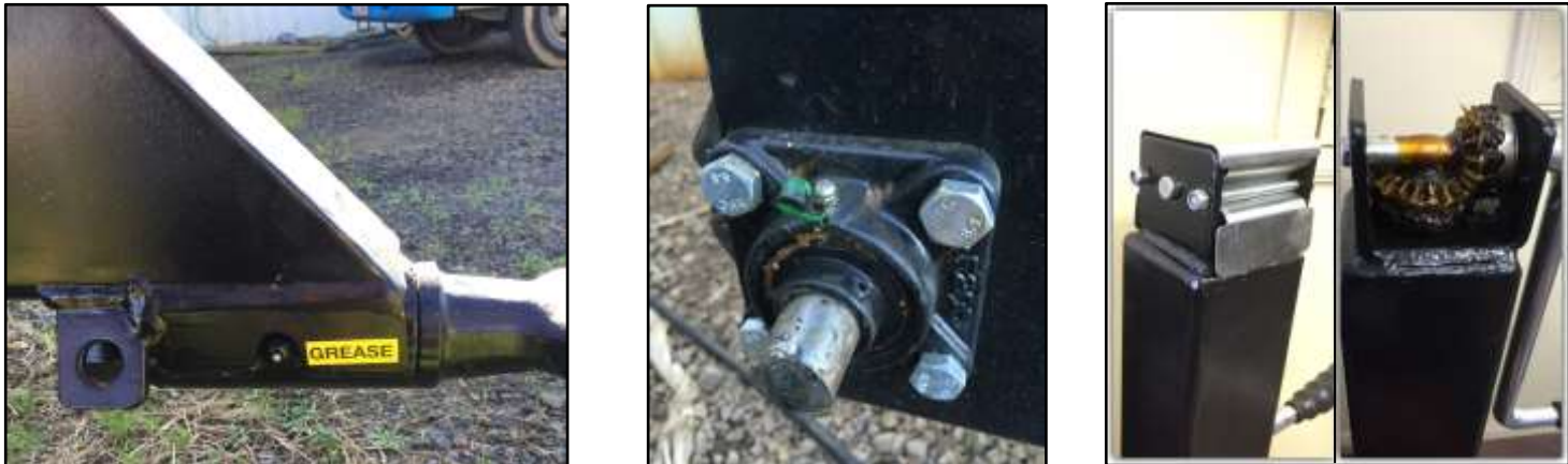
Pictured above is 1 of 4 bearings on sidefeed
